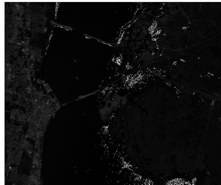
Fig. 17. Band 170 of KSC data set, from which lots of salt noises can be seen. In fact, this problem also occurs in many other bands.
